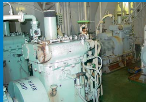
▶ Typical air compressors on a vessel
