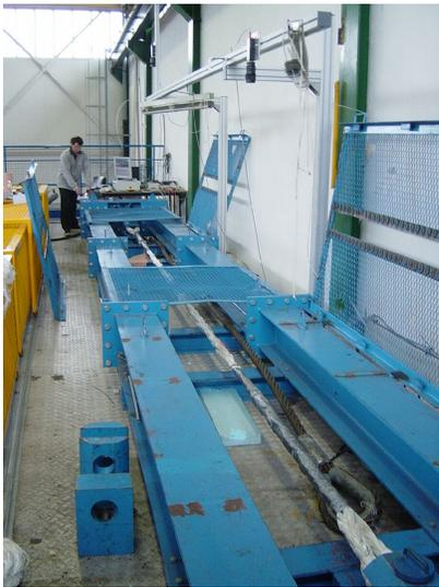
**Figure 1 . Sub-rope on test frame**
