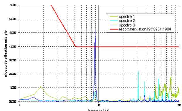
Figure 3 – Vibratory spectra and ISO 6954:1984 vibration level limit.
