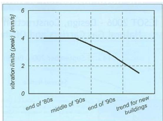
Figure 5 - Trends in vibration limits for passenger accommodation areas on cruise liner
