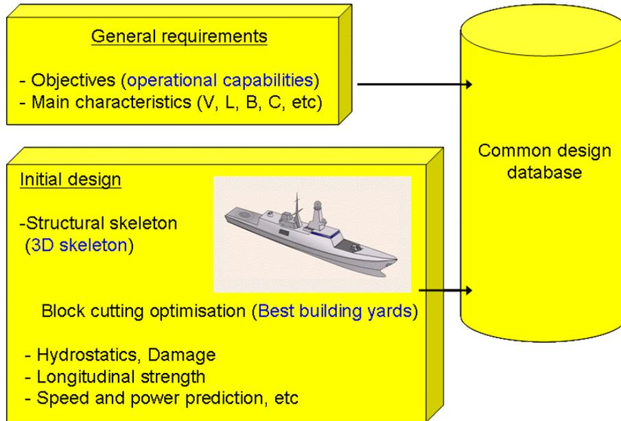
Fig.3: Common design - Requirements and initial design
