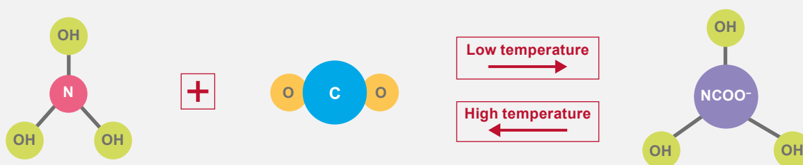
FIGURE 2.3: ABSORPTION AND SEPARATION PROCESS OF CO 2
